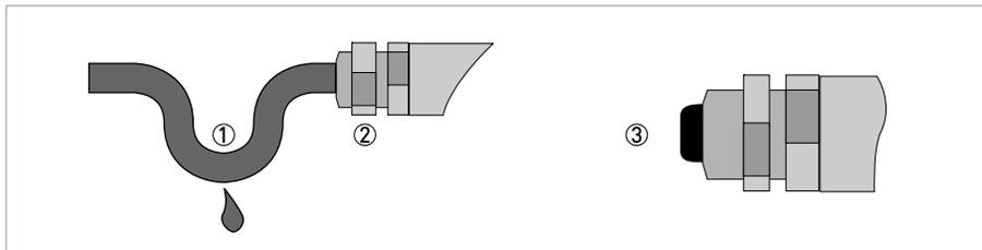
Figure 4-6: Protect housing from dust and water
