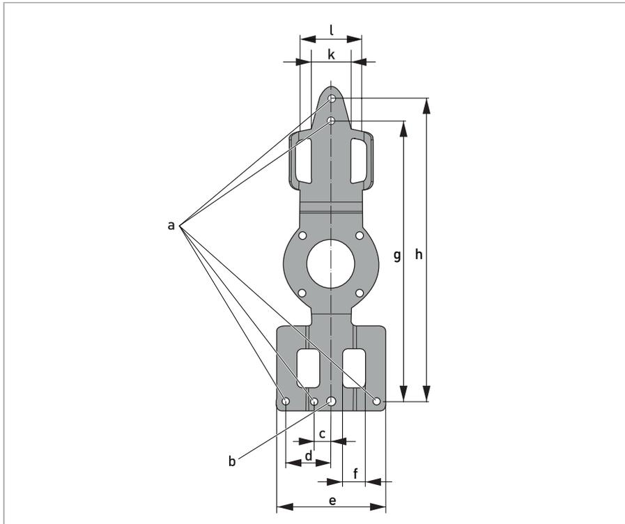
Figure 2-3: Dimensions of mounting plate, wall version
